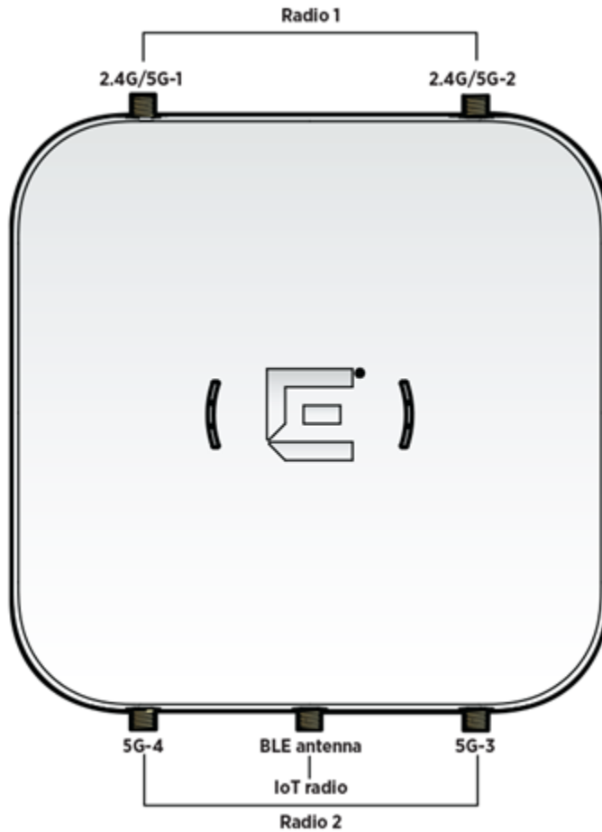
Figure 8: AP310e access point external antenna connectors
