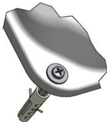
Figure 92: Self tapping screws inserted into the plastic wall insert plugs
